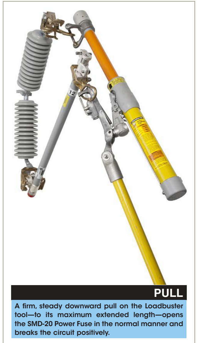
Figure 20. Load-current switching with the Loadbuster tool.
